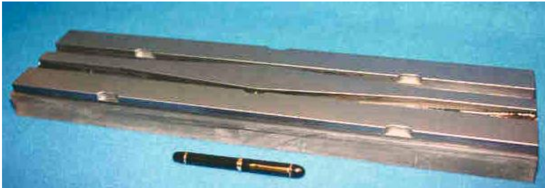
SILICON CARBIDE MIRRORS Length = 60 cm – Slope error = 0.5" RMS
