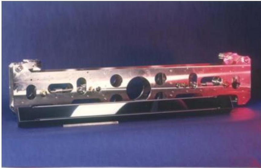
Example of 1.3 m silicon cooled mirror with its bender
